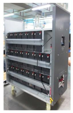
Remarks: to avoid short circuit, please be noted that the battery terminals must not contact the metal parts.
