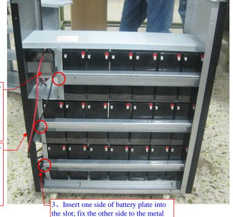
1. Insert one side of battery plate into the slot; fix the other side to the metal by M4\*8 screws.
