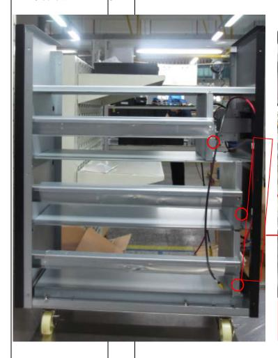
5. Paste the cable tie as shown in the picture. The opening of cable tie is outward.
